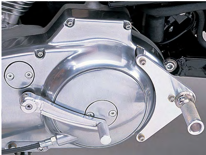
Left Side, 4 or 5 Speed, Reverse shift pattern 1986-2003
